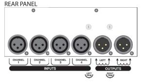
Mic Input: 1 - 4: XLR balanced inputs for connection to any standard dynamic or condenser microphone.
